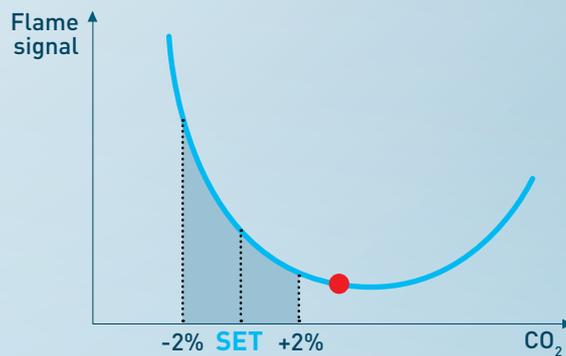
THE SYSTEM DETECTS THE DRIFT AND AUTOMATICALLY RUNS A NEW CALIBRATION TO GO BACK TO WORKING AT THE PRE-DEFINED SET
